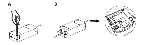
Insert the cable into the terminal block, then pull the cable lightly to make sure the cable is fi xed to the terminal block.
