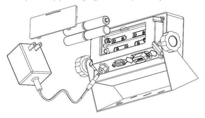
The INSTRUMENT may also be powered by the included AC wall adaptor.
