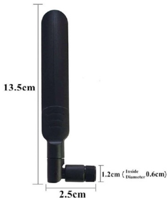
Figure 6: External Antenna Dimensions
