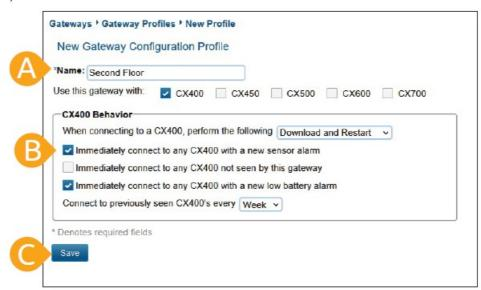
**Tip:** Refer to the full product manual for details on other configuration settings. Go to <a href="https://www.onsetcomp.com/intemp/resources/cx5000-manual">www.onsetcomp.com/intemp/resources/cx5000-manual</a>.
