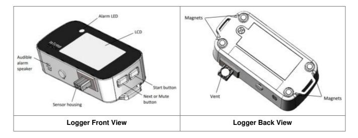
**Start Button:** Press this button for 3 seconds to start the logger when it is configured to start "on button push." You can also press this button for 1 second to bring the logger to the top of the list in the app. Press and hold both buttons on the logger simultaneously for 3 seconds to clear the minimum and maximum values on the LCD (see Minimum and Maximum Values) or for 10 seconds to reset a passkey (see Passkey Protection).
