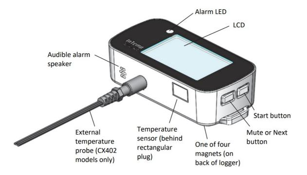
**Start Button:** Press this button for 1 second to start the logger when it is configured to start "on button push." Mute or Next Button: Press this button for 1 second to mute a beeping alarm (see Logger Alarms). For CX402 loggers, press this button for 1 second to switch between the external probe and ambient internal sensor
