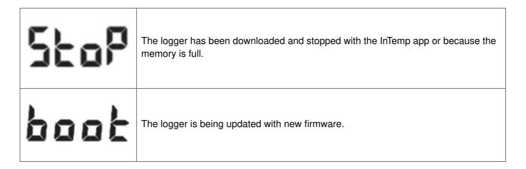
**Note:** If the logger has stopped logging because the memory is full, the LCD screen will remain on with "STOP" displayed until the logger is downloaded to your mobile device. Once the logger has been downloaded, the LCD will turn off automatically after 2 hours. The LCD will turn back on the next time the logger connects with your device.
