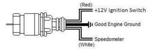
If replacing a cable: screw the provided sender onto the 7/8" male fitting you located previously for the existing electronic sender. If a two-wire sender, you should hook one of the two wires to the speedometer signal wire on the speedometer and the other wire to the ground.
