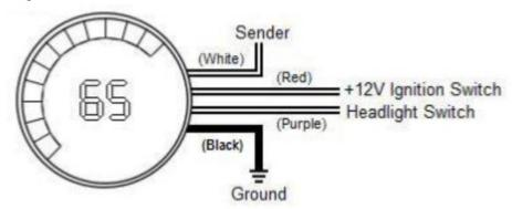
Power – **Red** Connect to a switched +12V source (such as the ignition switch)
