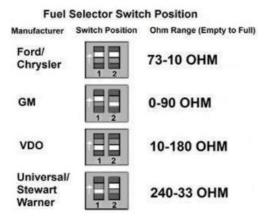
**Note:** FUEL GAUGE TEST The most common problem with our Fuel Gauge not working is the circuit is not complete. The easiest way to test this is to use a voltmeter and test for continuity on wires going to fuel sender. With wire disconnected from Fuel Gauge check for continuity to ground. Without this the Gauge will not work.
