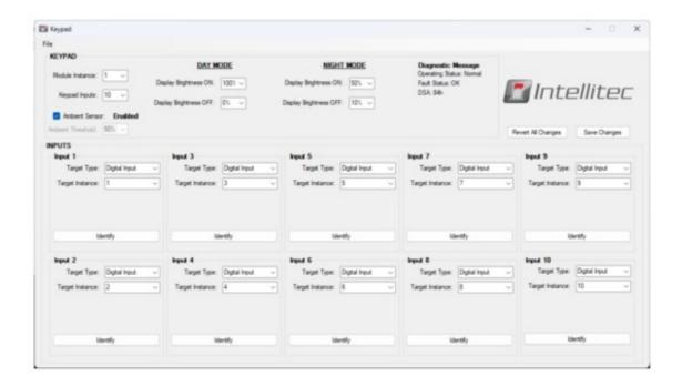
The RV-C Keypad GUI is a Windows-based tool that allows integrators to configure devices to their exact needs. This tool can configure all the parameters that are mentioned in the table above. Please note:
