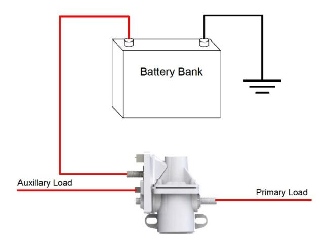
Wire Diagram 1 illustrates the primary connections of the Battery Guard® 1000. 5/16" bolts are used for the battery supply and Primary Load connections and are capable of supporting 100A of current. The Auxiliary Load uses a male 1/4" quick connect and can supply up to 2A of current to the Auxiliary Load.
