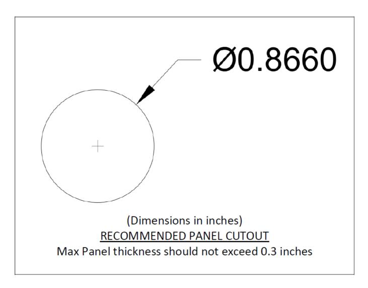
**Note:** Drawing dimensions refer to the switch used in the Intellitec kit (part # 10-01130-000). Installing the Battery Guard® 1000:
