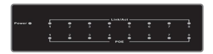
The LED indicators make monitoring and troubleshooting easier. If a status LED doesn't indicate a link or activity, check the corresponding device for proper setup and operation.
