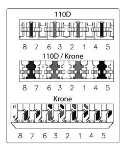
Refer to the IDC color codes on the back page to position each wire, and connect it to the patch panel using a Krone or 110D punch-down tool.
