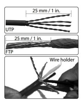
Strip away 25-30 mm of the cable jacket and separate the wires into 4 pairs. Cut the wire holder flush with the cable jacket.
