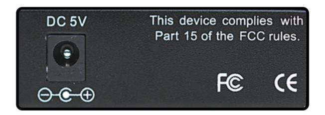
Plug the power adapter into the 5 V DC input jack on the media converter, then connect it to a regular power outlet. Only use the included power adapter or one with matching specifications (output of 5 V DC, at least 1 A).
