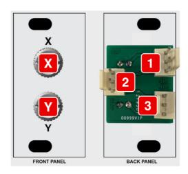
**[Y]** Y – This stereo 3.5mm (tip/ring/sleeve) jack, connects to **JP2 [2]** and JP3 [3] on the back panel as follows:
