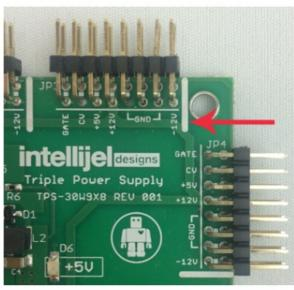
modules will come with the cable already connected but it is good to double check the orientation. Be aware that some modules may have headers that serve other purposes so ensure the cable is connected to the right one.
