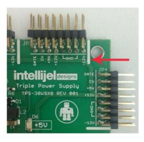
If you're using another manufacturer's power supply, check their documentation for instructions. Before reconnecting power and turning on your modular system, double-check that the ribbon cable is fully seated on both ends and that all the pins are correctly aligned. If the pins are misaligned in any direction or the ribbon is backwards you can cause damage to your module, power supply, or other modules.
