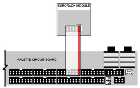
These are the the16-pin power connectors for powering your modules. The Palette 62 has 12 connectors, and the Palette 104 has 24. The connectors are shrouded to ensure that properly manufactured ribbon cables can be connected only one way — with the red (-12V) wire to the right.
