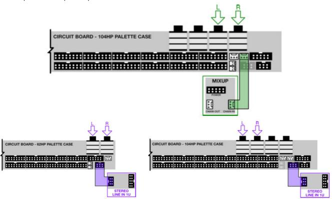
• Pedal I/O 1U: Connect the 3-wire link cable between the Link Connector on the Palette and the one on your Pedal I/O.
