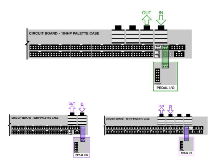
**IMPORTANT:** If you connect a module to the Audio Jacks Connector, you should not connect a module to the same audio pair's Link Connector (described later), or unexpected results may occur.
