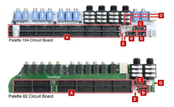
Running along the back edge of the Palette cases are their built-in circuit boards, which contain all of Palette's audio, midi, power, and module connection circuitry.
