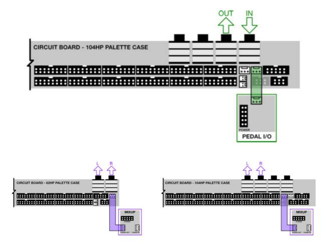
**Stereo Line-In 1U:** Using the cable provided with your Stereo Line In 1U module, connect it to the Audio Jacks Connector (or to one of the two Audio Jacks Connectors on the 104HP case). Once connected, the corresponding pair of Palette's TRS audio jacks function as L/R audio inputs for the Palette case.
