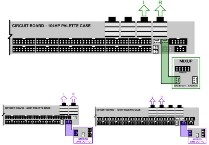
• Mixup (IN): Connect the 3-wire link cable (provided with your Mixup module), between the Link Connector on the Palette circuit board and the CHAIN-IN connector on your Mixup.
