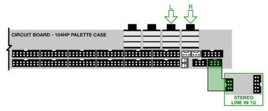
**IMPORTANT:** If you connect a module to the Audio Jacks Connector, you should not connect a module to the same audio pair's Link Connector (described later), or unexpected results may occur.
