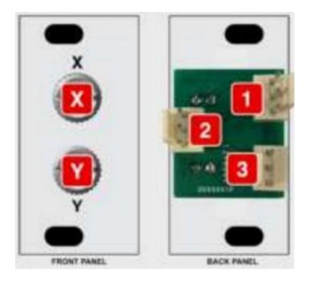
• X. X – This stereo 3.5mm (tip/ring/sleeve) jack connects to JP1 [1] and JP2 [2] on the back panel as follows:
