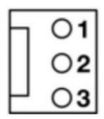
**Example 1: Mixup** – Connecting JP1 to the CHAIN IN on an Intellijel Mixup gives you an extra stereo input through the front panel **X** jack, where **X TIP** = **LEFT CH** of **Mixup**, and **X RING** = **RIGHT CH** of Mixup.
