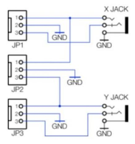
1. **JP1** – This 3-pin LINK connector is internally wired to the **X [X]** TRS jack on the front panel as follows:
