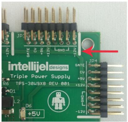
The other end of the cable, with a 16-pin connector, connects to the power bus board of your Eurorack case. Ensure the red stripe on the cable lines up with the -12V pins on the bus board. On Intellijel power supplies the pins are labeled with "-12V" and/or a thick white stripe, while others have shrouded headers to prevent accidental reversal.
