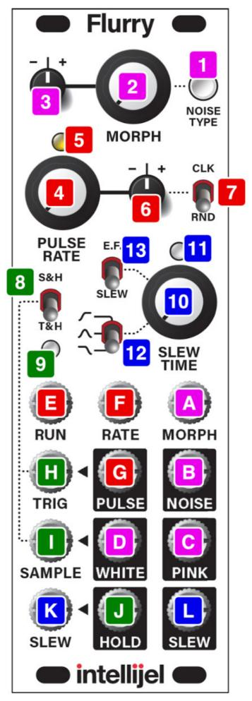
[7] CLK/RND switch - Sets whether or not the internal clock generates pulses at a steady, metrical rate; or whether it generates pulses at random intervals. The rate at which either mode generates pulses is set by the
