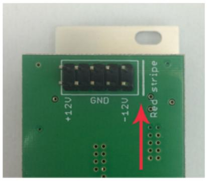
Ensure the 10-pin connector on the power cable is connected correctly to the module before proceeding. The red stripe on the cable must line up with the -12V pins on the module's power connector. The pins are indicated with the label -12V, a white stripe next to the connector, the words "red stripe", or some combination of those indicators. Some modules have shrouded headers to prevent accidental reversal.
