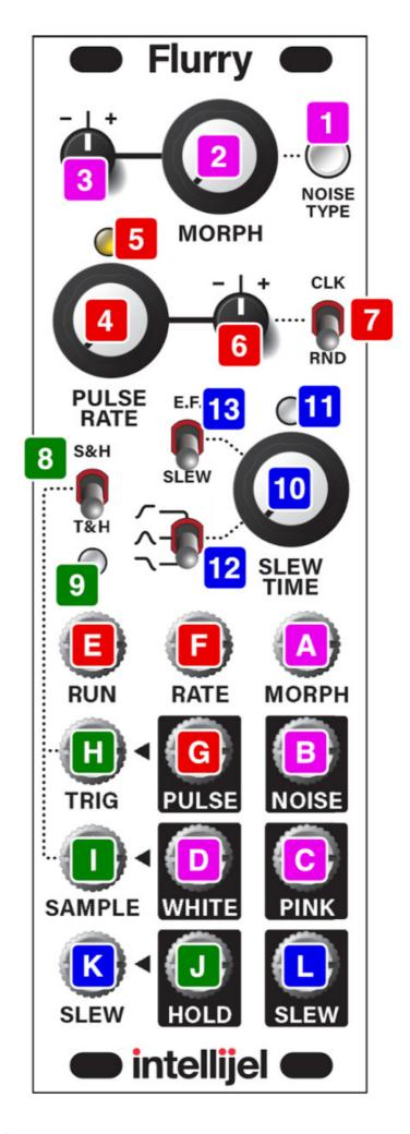
thus converting any instantaneous voltage changes appearing at the SLEW IN [K] jack to a gradual "slewed" voltage change at the SLEW OUT [L] jack.
