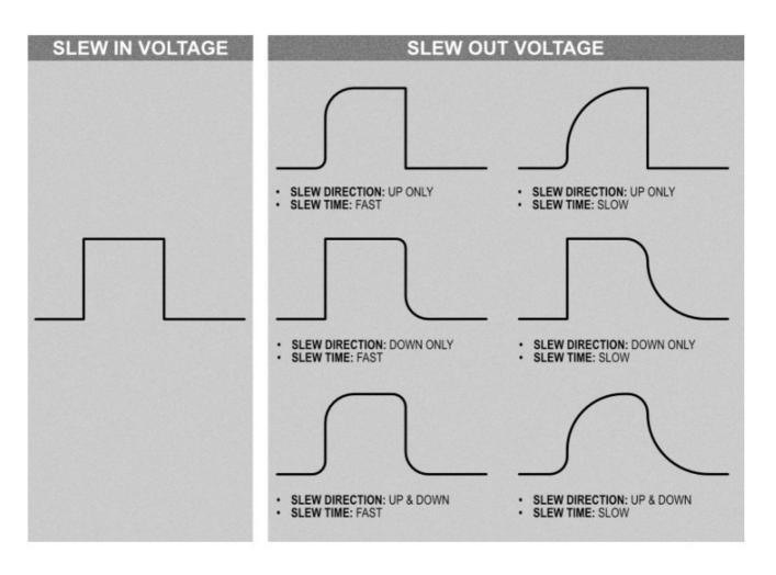
[13] SLEW / E.F. switch – Sets whether the slew circuit functions as an envelope follower (E.F.) or as a standard slew. Specifically:
