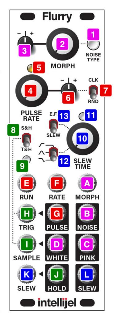
• S&H (up): Flurry operates as a traditional sample & hold — sampling the SAMPLE IN [I] voltage at the rising
