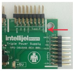
Most modules will come with the cable already connected but it is good to double check the orientation. Be aware that some modules may have headers that serve other purposes so ensure the cable is connected to the right one.
