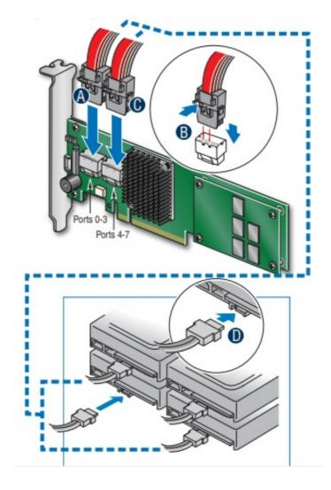
Rear view of four SATA drives connected to ports 0-3 on the Intel® RAID Controller RS25DB080
