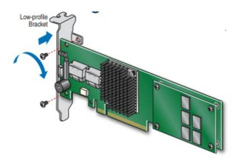
E Replace and tighten the two screws.
