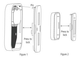
The sensor must be installed according to the images below, with the magnet aligned with the sensor body and with the smallest possible distance between them, so that the magnet is in contact with the magnetic field sensor.
