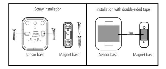
**Important** check if the GAP distance (distance between the sensor and the mag-net) is within the specification, to avoid unwanted triggering in case of any vibration in the structure where the sensor is installed. **Note** the type of surface where the sensor is installed may influence the distance from the GAP.
