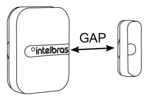
To close the sensor, check the pin located on the base, it must be positioned on the same side as the battery, after positioning the base, just press it for locking, there is only one way to close the sensor, check image 01 To close the magnet, just position the base and press it, image 02.
