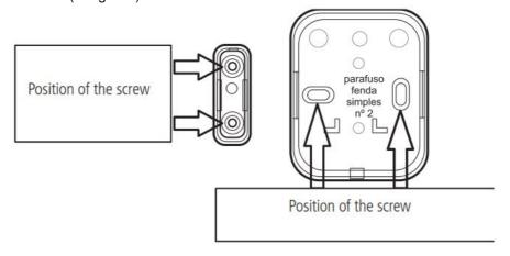
The sensor must be positioned as shown in the figure, so that the magnet is in contact with the SMD Reed Switch. **Note**: for closing and opening the SMD Reed Switch, some average distances must be respected.
