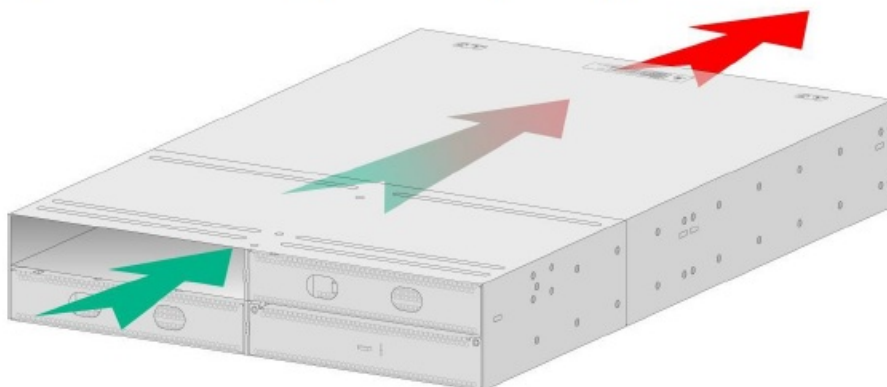
Figure4-1 Airflow from the port side to the power supply side through the device chassis
