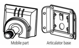
**Attention**: if the mounting bracket is inclined with respect to the ground, the characteristics of the PET function will change.
