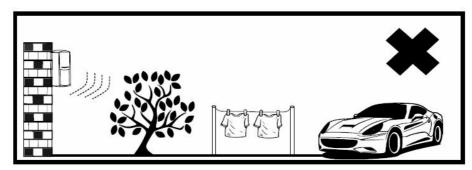
• Do not use the sensor in areas with sudden changes in temperature, near air conditioners, heaters, cooling fans, and ovens.
