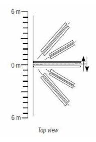
• Do not place objects in front of the sensor. Keep the detection area free of moving objects, bushes, clotheslines, cars, or any object that blocks the scan. Do not exceed the maximum sensor installation height (2.4 m).
