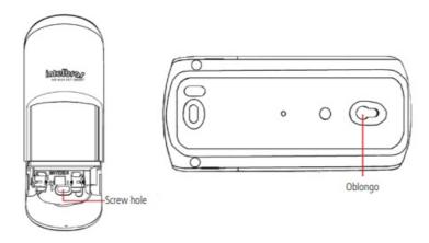
• Step 3: if the installation is done in the corner of the wall. Use the holes indicated on the back cover.
