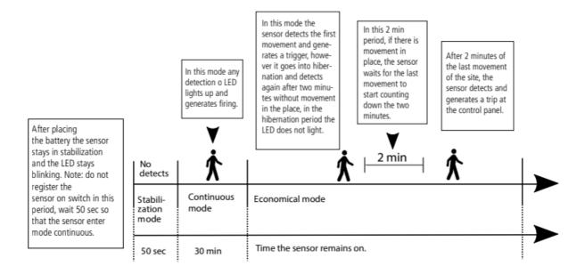
With jumper JP2 open, the sensor will work in CONT (intelligent continuous) mode, operating as follows: After power-up, the sensor will work continuously for 30 minutes so that the installer can make all the adjustments to the sensor.
