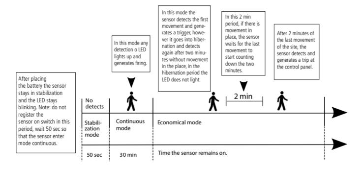
After power-up, the sensor will work continuously for 30 minutes so that the installer can make all the adjustments to the sensor.
