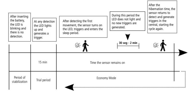
**Advantage of the Economy mode:** this ability to learn from the environment, means that in places with high degrees of movement, periodic and non-continuous shots are generated, in turn, saving battery power.
