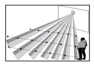
If the alarm control panel used is Intelbras, put it in test mode, this way it will not be necessary to observe the LED, as the control panel will indicate the sensor's operation through siren beeps.
