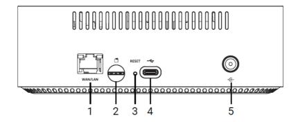
The rear of the GX 1001 LT has the following connections.
