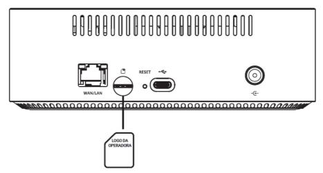
**Note**: to access the internet, you can also connect a network cable to the WAN/LAN port of the GX 1001 LT and the other end of the network cable to the internet modem or DHCP server.
