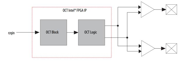
The OCT Intel FPGA IP allows you to dynamically calibrate I/O with reference to an external resistor. The OCT IP improves signal integrity, reduces board space, and is necessary for communicating with external devices such as memory interfaces. The OCT IP is available for Intel Stratix® 10, Intel Arria® 10, and Intel Cyclone® 10 GX devices. If you are migrating designs from Stratix V, Arria V, and Cyclone V devices, you need to migrate the IP. For more details, refer to the related information.
