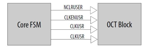
The Fitter does not infer a user-mode OCT. If you want your OCT block to use the user mode OCT feature, you must generate the OCT IP. However, because of hardware limitations, you can only use one OCT IP in user mode OCT in your design.
