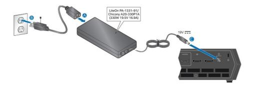
Each Intel NUC model includes either a region-specific AC power cord or no AC power cord (only the power adapter).
