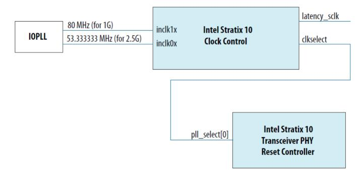
You must ensure that the inclk0x port connects to 2.5G sampling clock and the inclk1x port connects to 1G sampling clock. The output clock port of clock control becomes the latency\_sclk port. For design migration from the Intel Arria 10 devices to the Intel Stratix 10 devices, you can reuse the similar connectivity between the 1G/2.5G reconfiguration block and transceiver reset controller.
