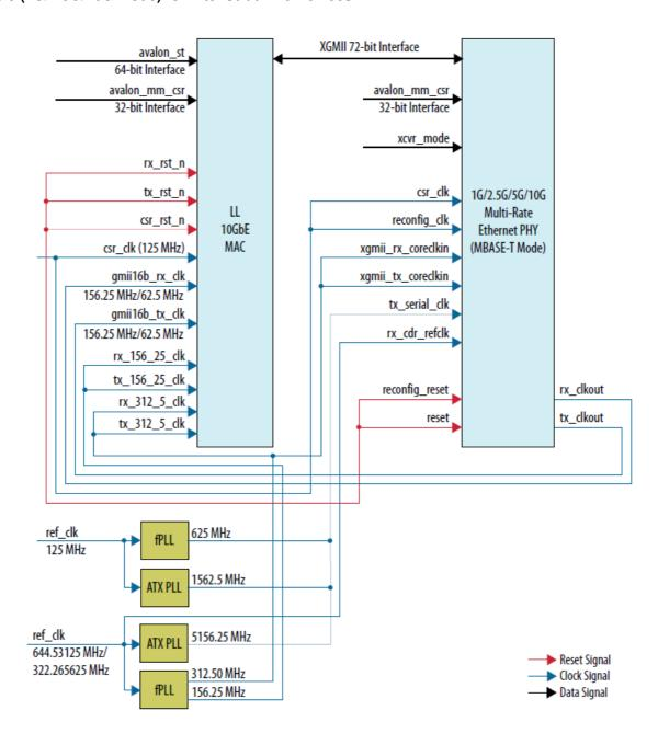
The following figure illustrates the latest clocking and reset scheme of the 1G/2.5G Ethernet with IEEE 1588v2 feature design example targeted on Intel Stratix 10 devices. There are differences between this solution and the version that was introduced in the Intel Arria 10 devices. Modification is needed when migrating design from the Intel Arria 10 devices to the Intel Stratix 10 devices.
