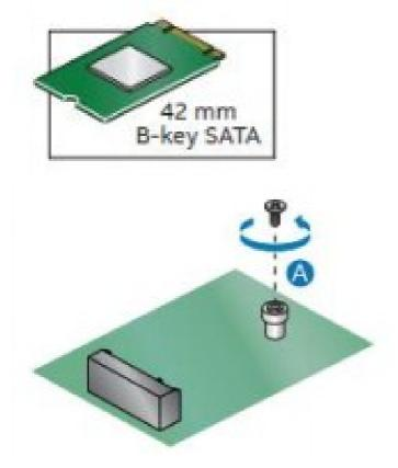
2. Move the standoff (B) from the 80mm position to the 42mm position (C).
