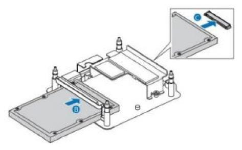
2. Secure the drive into the drive bay with the two small silver screws that were included in the box (B). Set the drive bay bracket down inside the chassis (C).
