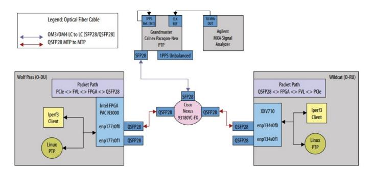
The PTP4I output on each of the DUT hosts provides data measurements of the PTP performance for each slave device in the setup (Intel FPGA PAC N3000 and XXV710). For iperf3 traffic test, the following conditions and configurations apply to all graphs and performance analysis:
