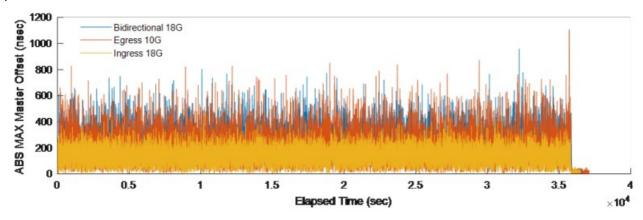
The following figure shows the mean path delay for for XXV710, under ingress, egress and bidirectional iperf3 traffic.
