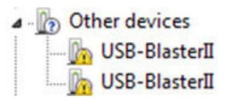
You need to install drivers for each interface: one for the JTAG interface and one for the System Console interface.
