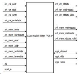
Figure 1. Ports Block Diagram
