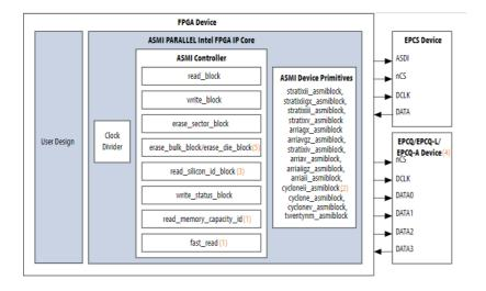
The ASMI Parallel II Intel® FPGA IP provides access to the Intel FPGA configuration devices, which are the quad-serial configuration (EPCQ), low-voltage quad-serial configuration (EPCQ-L), and EPCQ-A serial configuration. You can use this IP to read and write data to the external flash devices for applications, such as remote system update and SEU Sensitivity Map Header File (.smh) storage.
