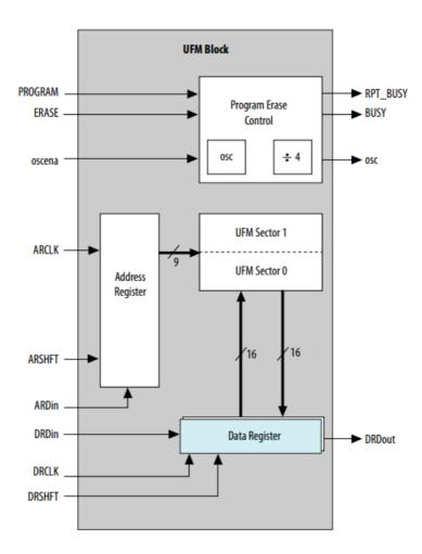
The internal oscillator is part of the Program Erase Control block, which controls the programming and erasing of the UFM. The data register holds the data to be sent or retrieved from the UFM. The address register holds the address from which data is retrieved or the address to which the data is written. The internal oscillator for the UFM block is enabled when the ERASE, PROGRAM, and READ operation is executed.
