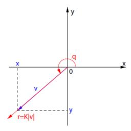
The function takes inputs x and y and outputs a=atan2(y, x) and M = K(x2+y2)0.5. M is the magnitude of the input vector v=(x,y)T, scaled by a CORDIC specific constant that converges to 1.646760258121, which is transcendental, hence has no fixed value. The functions supports two configurations, depending on the sign attribute of x and y:
