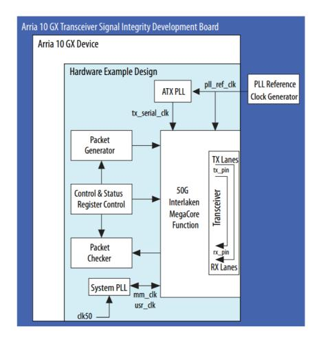
The hardware example design includes external PLLs. You can examine the clear text files to view sample code that implements one possible method to connect external PLLs to the 50G Interlaken IP core.
