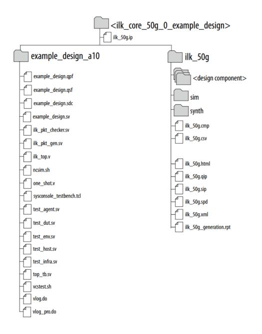
The hardware configuration, simulation, and test files are located in <example\_design\_install\_dir>/example\_design\_a10.
