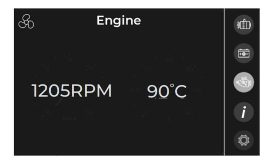
The system indicates if the engine is in or out of gear. The gear status is displayed at the top left with a propeller
