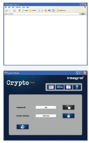
You are now ready to use the Crypto Dual drive. All data that is put in the secure partition will be fully encrypted automatically, or by locking the device via the lock icon or after removing the USB Flash Drive from the socket or if there is a suspension of power. Access to this is only granted with the correct password.
