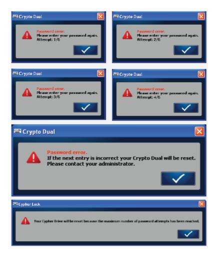
At this point the Crypto Dual drive is not usable until the Dual Lock application has reset. At this stage the drive will be reset back to factory settings and you will see a confirmation message when it is done.
