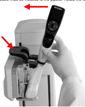
housing of the pipette by 90 degrees as displayed in the picture below.
