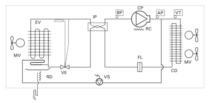
CP: COMPRESSOR MV: MOTOR FAN EV: EVAPORATOR CD: CONDENSER
