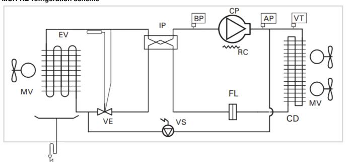
CP: COMPRESSOR MV: MOTOR FAN EV: EVAPORATOR CD: CONDENSER
