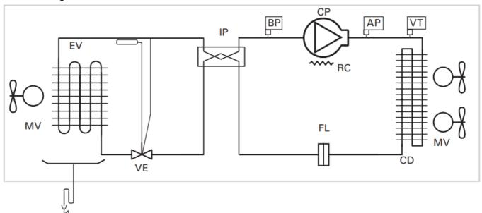
CP: COMPRESSOR MV: MOTOR FAN EV: EVAPORATOR CD: CONDENSER
