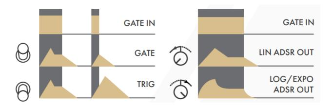
A trigger signal at the Gate/Trig Input (or a gate signal with a duration shorter than the attack and/or decay stages), will force the envelope to prematurely jump to the release stage.
