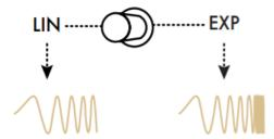
• If the toggle is set to exponential FM and the FM Attenuator is fully clockwise, the FM Input will essentially track at 1V/Octave (Its tracking may differ slightly from the calibrated 1V/Oct Input).
