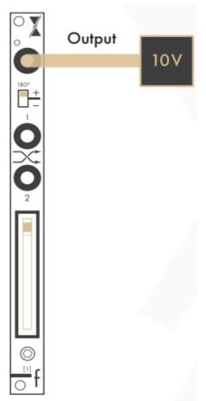
Unipolar Negative DC Offset: If no signal is present at the Inputs and the Polarity Switch is in the down position, the module acts as an unipolar negative DC offset. When the Fader is in the highest position, -10V is generated at the Output. Moving the Fader downwards attenuates the DC offset down to 0V at the lowest Fader position.
