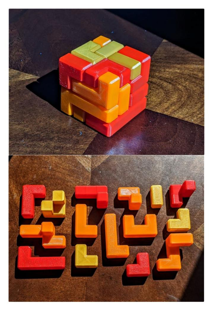
I printed all of the pieces in PLA with 5% infill, although 10% is probably ideal. All but one of the pieces can be 3d printed without supports. The piece that needs support is shown in the upper right of this step.
