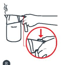
Press pouring release button for several seconds, then pour and discard water.
