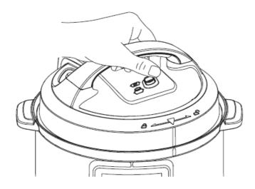
2. Turn the lid clockwise until the line on the lid lines up with the line on the control panel.
