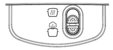
2. When pressure is released, the steam icon on the display OK to Open Lid, remove the lid.
