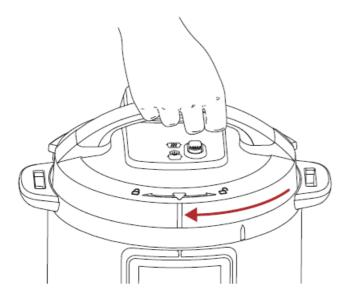
If the lid is not closed and locked when you start a cooking program, the message display will show Turn to Lock Lid and the unit will not start pressurizing.
