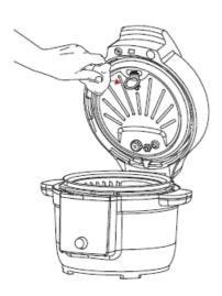
3. Press the red button on top of the lid, and the Inner Cover will release.
