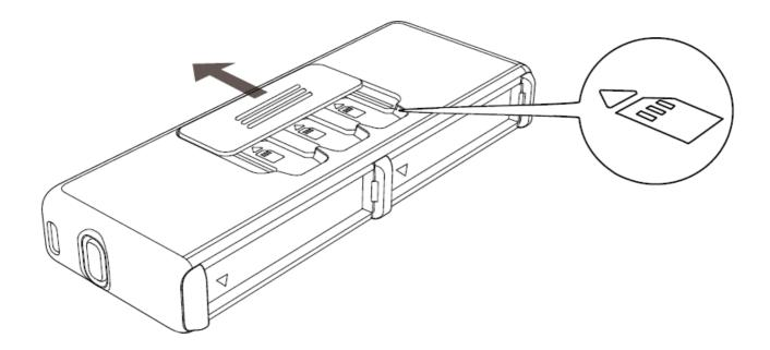
Remove the cover on the back of the Utility Fast Charge Case and insert microSD cards as shown. The case can store up to three microSD cards at once.
