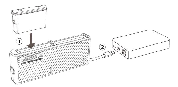
1. Align the notch of the battery with the triangular mark on the battery slot, then insert.
